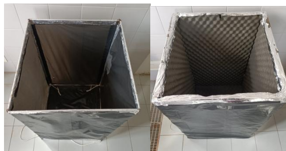
Fig.1. Prototype of the nylon (left) and steel (right) boxes used in the reported experiments, seen from the bottom side.
